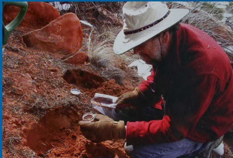
Soil sampling for geochemical analysis in the Lisbon field area of the Paradox Basin. Geochemical surveys analyze soil samples for trace amounts of hydrocarbons that have naturally seeped to the surface from undiscovered oil traps.
